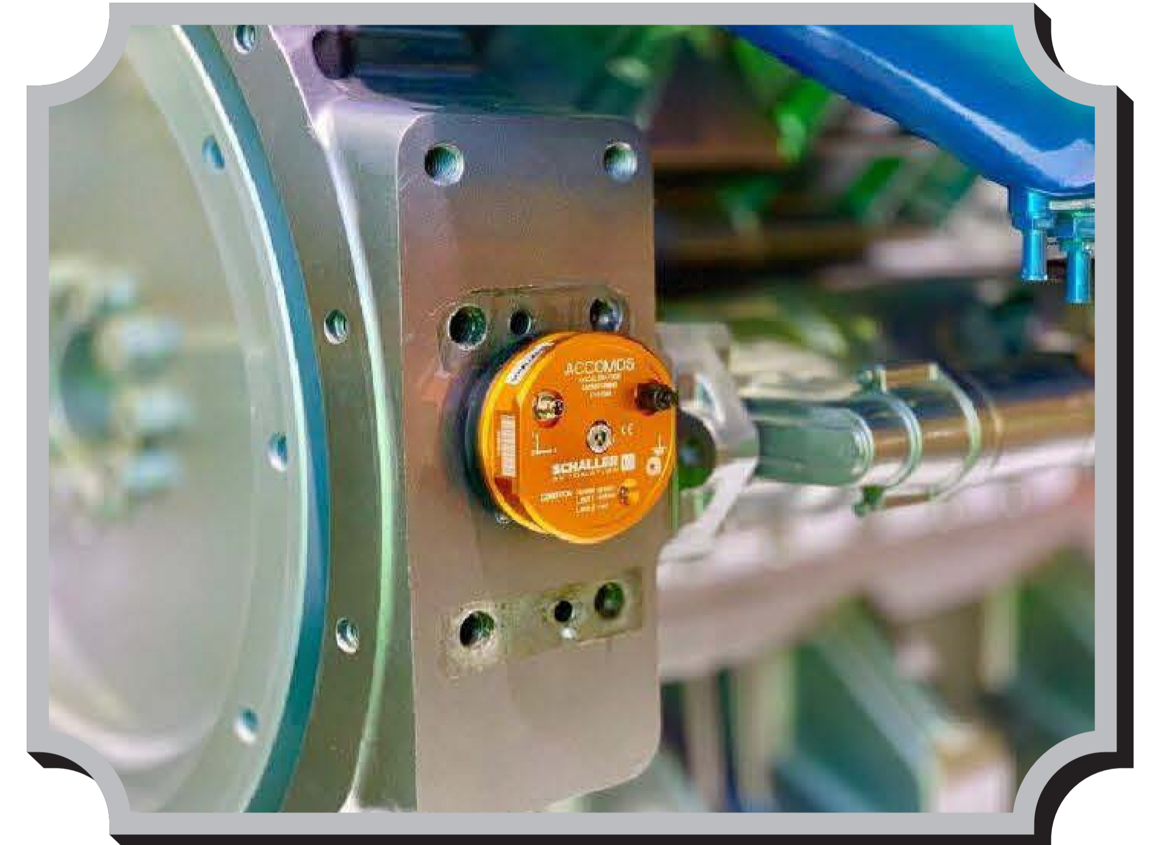
SCHALLER ACCOMOS® VIBRATION MONITORING SYSTEM
