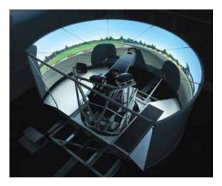
Simulators are increasingly used in professional motorsports for driver training and vehicle development. The sophistication of such simulators is rapidly improving to provide a complete, realistic driving experience with visual, audio and – importantly – motion feedback to the driver.
