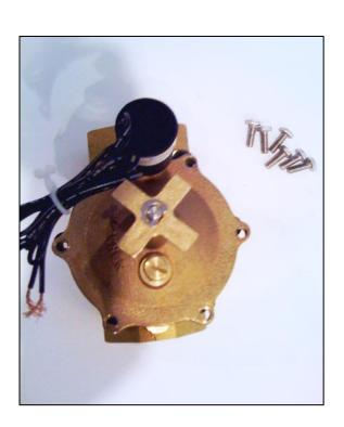
**2.** Lift bonnet assembly off of valve body.
