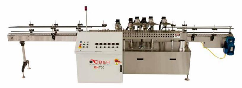
THE BH700, when paired with any BH or Marathon roll-fed labeler, creates a durable and dependable roll-on shrink-on labeling system. Based on the industry standard B & H Endura® Process, the BH700 provides high-impact shrink labeling at a lower cost versus shrink sleeve labeling.
