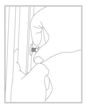
d. Insert the holding nut, bolt and 2 washers and hand tighten.
