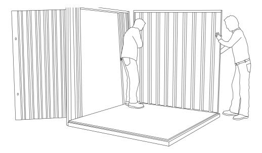
b. The wall panels should inter-lock.
