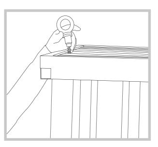
f. Outside attach the lifting eyes (with their rubber washer) to the end of the lifting rods.
