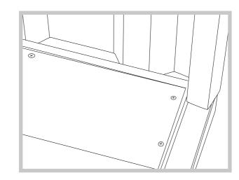
c. Butt the panel up against the chassis edge.
