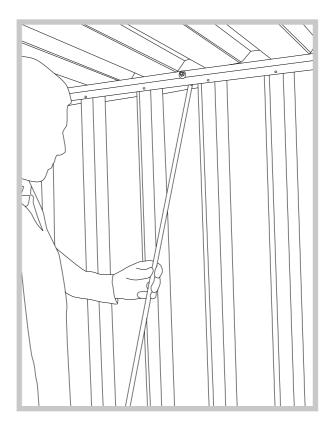
d. Inside insert the 4 lifting rods through the eyelets at the top and into the captive nuts in the chassis.
