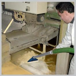
Vacuum cleaning in animal feed mixing plants with stationary and mobile vacuum systems.
