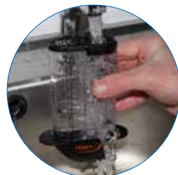
Measure water flow of domestic appliances to ensure a sufficient flow rate.
