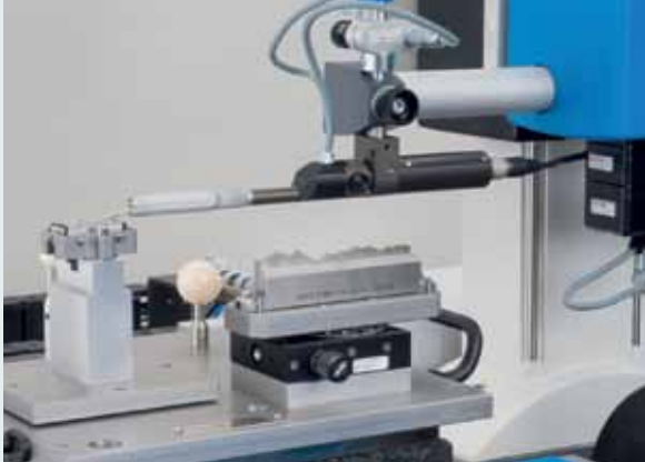
The calibration of the measurement system is automated via integrated roughness and contour standards.
