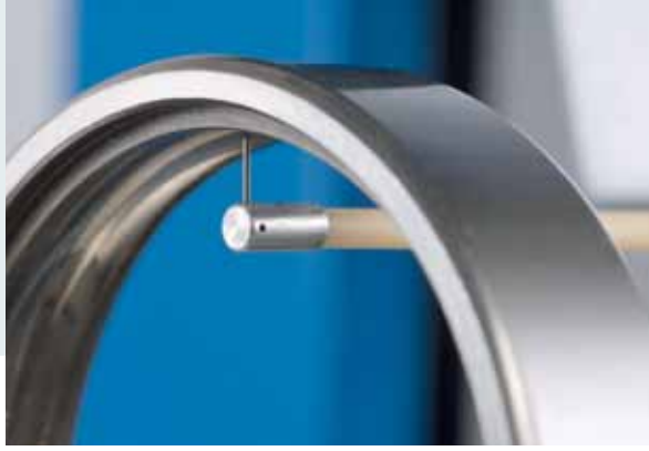
Combined roughness and contour measurement
