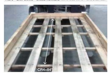
FIG. 6 – LAM-CRATE – CROSS RUNNERS Underside view with 84" forks
