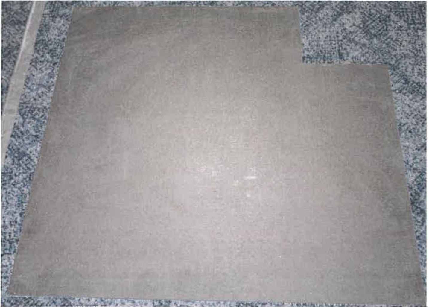
Image 1: Laminam 5.6 mm prior to testing.
