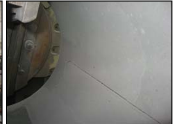
Body being rebuilt and machined with Belzona 1311
