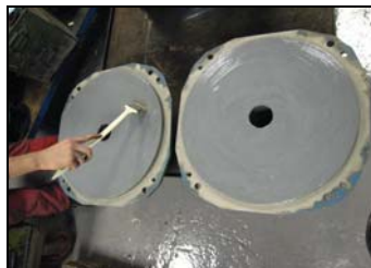
Rotor and end coated with Belzona1341
