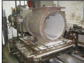
Body being rebuilt and machined with Belzona 1311
