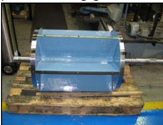
Rotor and end coated with Belzona1341
