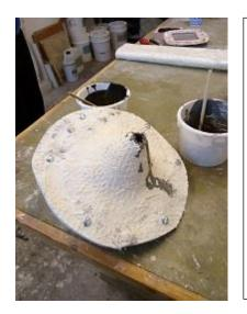
Jesmonite AC 300 laminated 2 part mould jacket over a silicone mould for slush moulded polyester ball.
