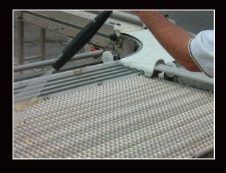
The stainless steel Easy Clean™ conveyor design integrated with the anti-microbial roller surface, inhibits the growth of bacteria, mold and other unwanted organisms, netting a cleaner conveyor system.
