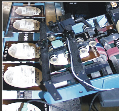
►► The ejection carriage creates a perfect separation for single shot or batch counting
