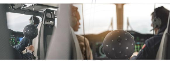
TotalSim are happy to help with reducing your noise problem. The acoustic camera can be placed in a vehicle (for example a car, yacht or train) to show the location of the dominant noise sources. Since the capture and analysis is very quick it is possible to test different noise reduction strategies within the same session. The output from the camera will show which strategy is most effective in reducing the noise and improving passenger comfort.
