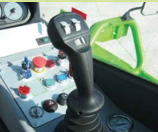
The electro-mechanical joystick gives the operator full control of boom and upperstructure in one lever.
