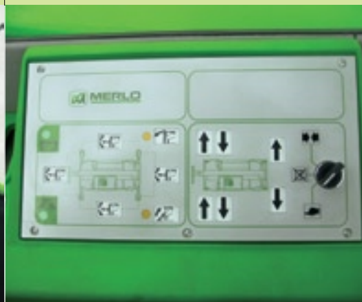
Controls for the stabilisers and suspension (S models) have been regrouped into a wide lateral console.
