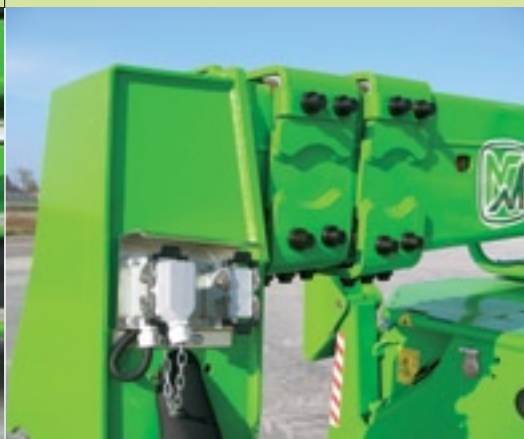
Boom sections slide on adjustable low-friction pads.
