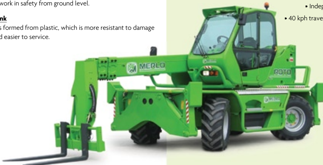
The four stabilisers legs when retracted lie within the width of the machine.
