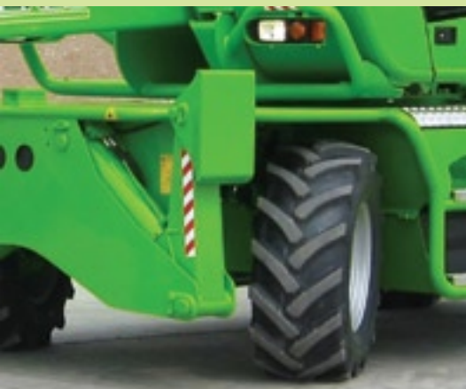
The four stabilisers legs when retracted lie within the width of the machine.
