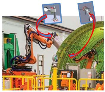
Unlike metal riveting tools which have progressed from manual to automated installation, adhesive bonded fixings are still primarily manually installed.
