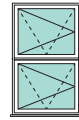
Desripton: R/H OPENER WITH TILT OVER R/H OPENER WITH TILT Code: SIG700
