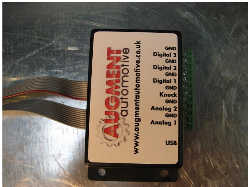
Figure 7: Breakout Box Top View
