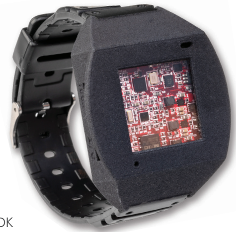
Chilkat HDK comes with a wrist-worn strap for easy data collection and testing of the AI models.
