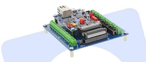
CNC310 with DIN Rail Mount and Breakout Board:
