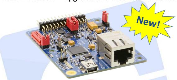
The smallest CNC controller from Eding CNC. This controller controls up to 3-axis with a 125kHz step frequency via its USB interface with Eding CNC Starter Software. This enables you to do 2.5D CNC operations. But wait...you need more?
