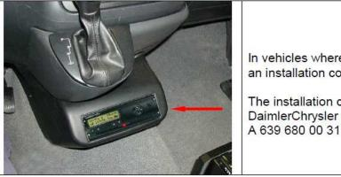
In vehicles where both radio compartments are occupied, an installation console can be mounted.
