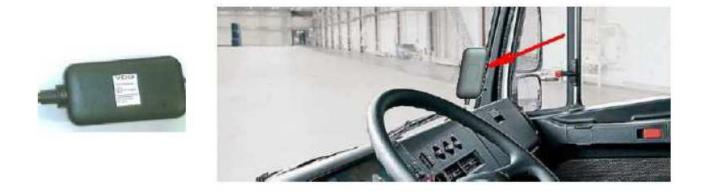
Please Note: The Geoloc is equipped with a 120 Ohm Can Resistor. The CAN wiring to CAN1 or CAN2 must take this into account!
