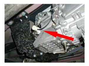
Locate blanking plug, remove and install sender unit supplied
