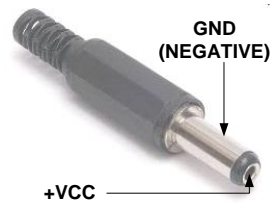
Figure 13. How the power supply cable must look like
