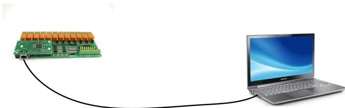
Figure 16. Connecting DAEnetIP4 12 Relay Module to a computer directly (recommended initial connection)
