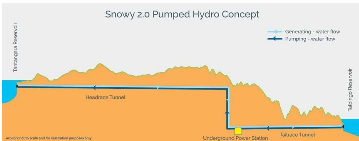
Figure 1 Conceptual design for Snowy 2.0 Source: Source: Snowy Hydro
