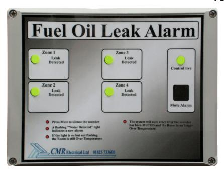
The ODS4 has been designed to monitor four independent zones for fuel oil leaks including but not limited too, Diesel, Heating and Hydraulic oils via optical sensors.
