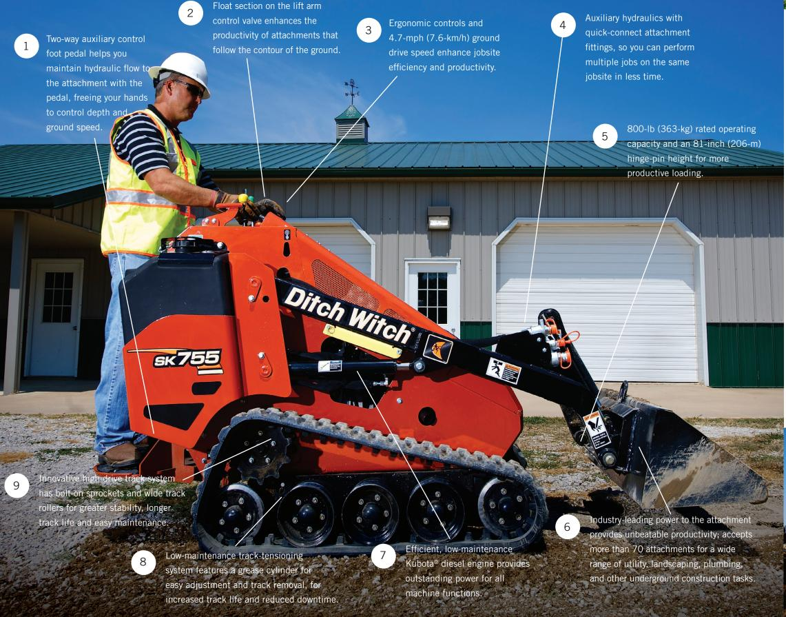
The Ditch Witch® SK755 Mini Skid Steer is built to outperform on any jobsite. Featuring a high-drive track system and an enhanced operator's station, it delivers superior performance through increased ground clearance, more lift capacity, faster ground speed, longer track life, and more operator comfort. And with more horsepower to the attachment than the competition, the SK755 will help make you more productive and more profitable, job after job.
