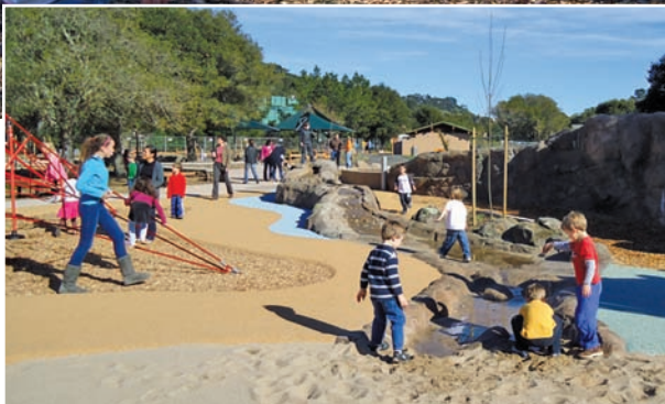
Above: The toddler makes a break for it! The renovated park includes expanded picnic areas with new recycled plastic picnic tables and steel trash receptacles (both from Dumor Site Furnishings). The surfacing is decomposed granite with a resin binder to create an accessible surface.
