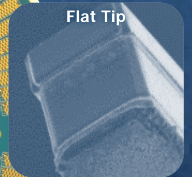
40µm pitch MEMS probe tip grid array
