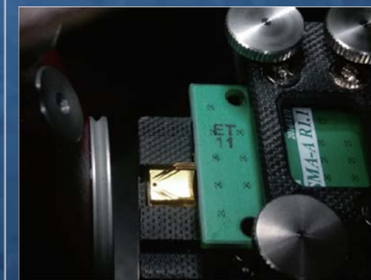
Edge Emitting Device Testing
