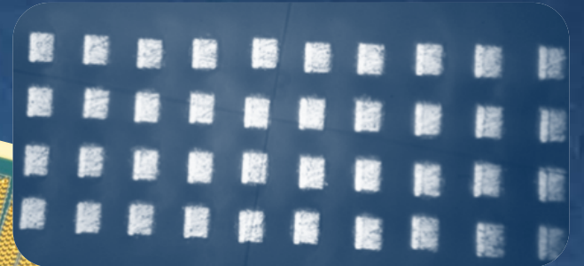
40µm pitch MEMS probe tip grid array
