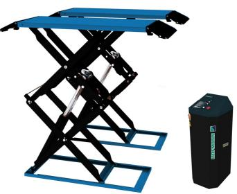
A pneumatic safety locking system and drive-on ramps which can be used as platform extensions are additional features of the SSL 3000, which comes with an air connector/lubricator and four rubber blocks as standard accessories.
