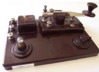
Blue Point key, buzzer and light set.
