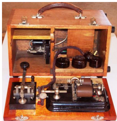
P.M.G. Portable set (key, relay and sounder). Pre set up.
