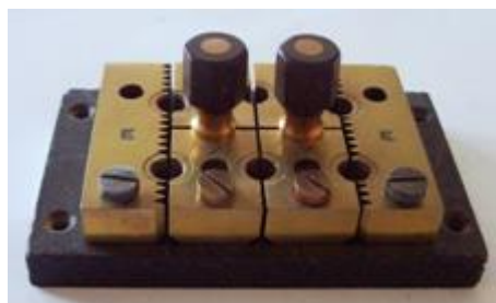
P.M.G. Section switch. (Used mainly in Victoria)
