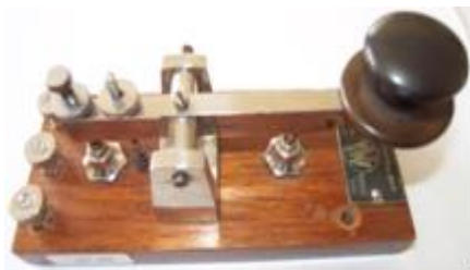
A.W.A. R688B. A similar key was made by Cinema Engineering P/L. The label read 'Type Like R688B Manipulating Key Cinema Engineering Pty Ltd'. The knob was embossed 2018 A2-14. Similar key also made by A.V. Sales Pty. Ltd.
