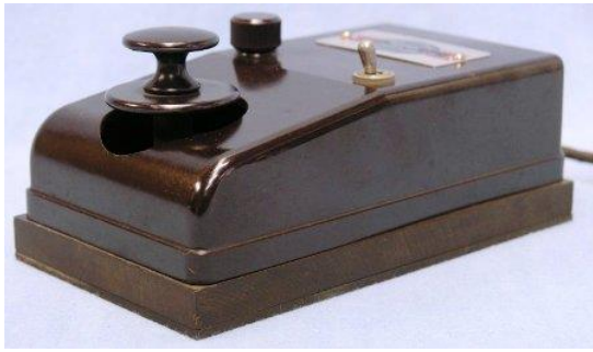
Military key made by Weston Electronics Sydney. Very similar to UK RAF Type D except for switch.
