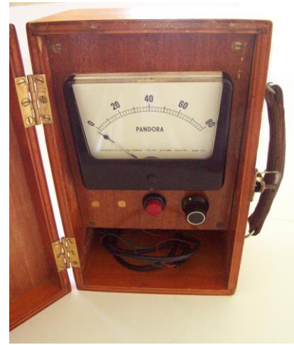
'Pandora's Box'. Used for testing underground cables.
