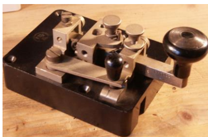
P.M.G. Workshops modified WT8amp key. (Round corner model)
