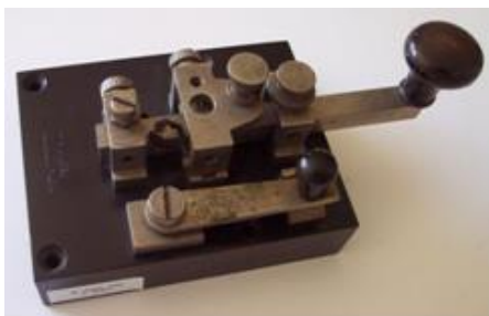
P.M.G. Workshops modified WT8amp key. (Square corner model)
