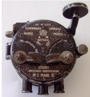
Military key made by Weston Electronics Sydney. Very similar to UK RAF Type D except for switch.
