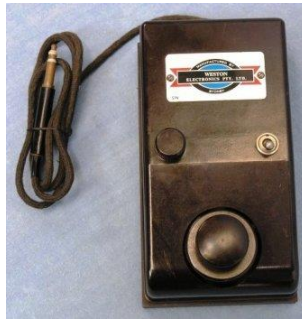
Military key made by Weston Electronics Sydney. Very similar to UK RAF Type D except for switch.
