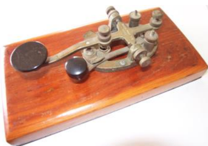
Buzza U.S. design straight key.
