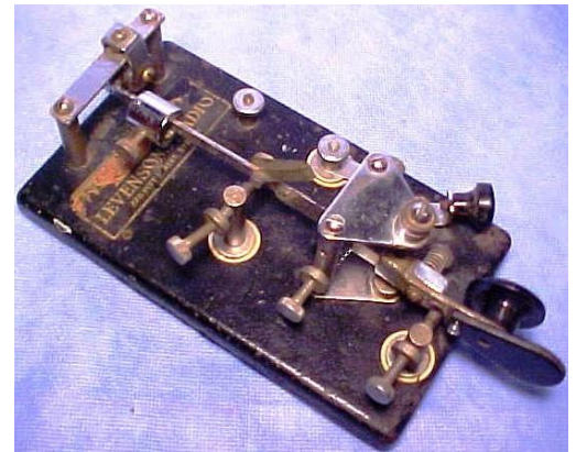
Levenson 'Like A Flash' semi automatic key (Almost certainly made by Buzza).
