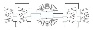
number of directions. In a general arable situation the slave units give valuable extra protection when directed towards peripheral trees/power lines where birds tend to perch before feeding. Slave units are available as end units with one socket or intermediate units with two sockets.
