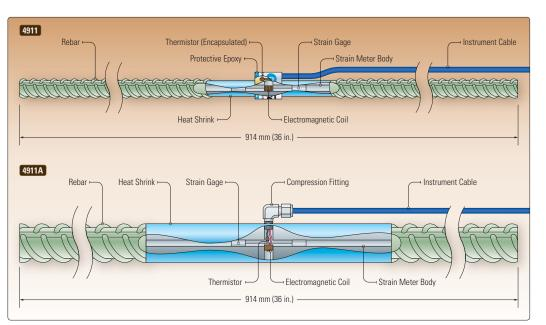
• Illustration of the Model 4911 "Sister Bar" and Model 4911A Rebar Strainmeters and their various components.
