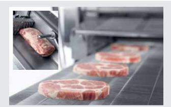
Single slice weighing: each slice is cut between 50 and 300 g target weight, with deviations in even or slightly bulky products at only about 4 %. This drastically reduces giveaway.
