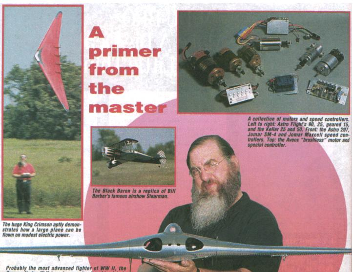
German Horten IX flying wing was developed too late to see action. This ducted-fan model uses twin, homemade 2%-inch rotors turning at 32,000rpm to create 48 ounces of thrust.
