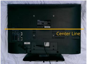
2. Measure from the center line to the center of the top left mounting hole, and note this distance down.
