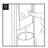
When the external cleaning (minimum 5 minutes) is completed, flush the machine using the chilled button with clean water until the dispense water runs clear. Repeat briefly with the ambient button.
