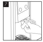
Leave the solution inside machine for sanitisation (minimum 5 minutes) while thoroughly cleaning the machine externally, pay particular attention to the dispense faucet and buttons.
