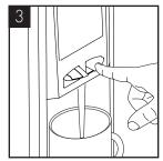
Dispense chilled water until the baffle plate is accessible.
