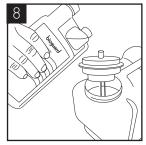
Remember to include the drip tray. If a Waste Overflow System is fitted, empty this and flush through with a small amount of sanitisation fluid if needed.
