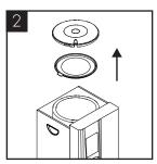
Remove the polystyrene lid. Gently lift the plastic lid from the tank, taking care not to disconnect the plumbing.
