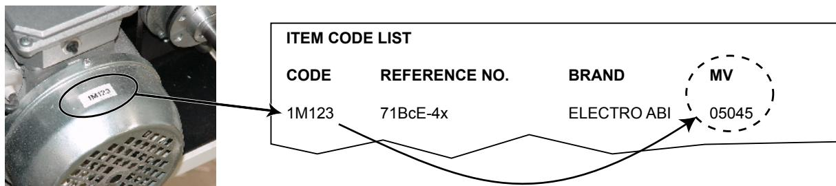
The code number may also be found on the electrical diagrams and in the code/function list. The latter contains a description of the part in question (see separate diagram book).
