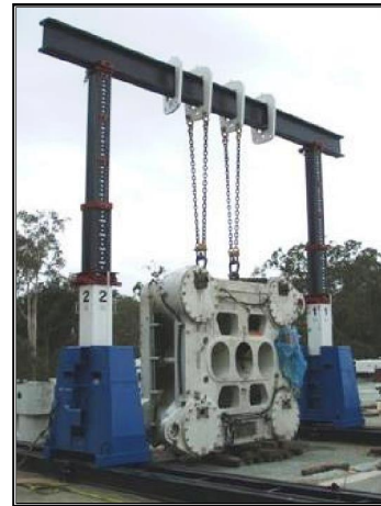
J&R L1001-2-34 LIFT-N-LOCK hydraulic boom gantry project in Brisbane, Australia.
