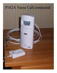
For bed vacation the unit is best positioned about 2 m from the bed and set on the floor. Normal movement around the bed will go undetected but once a foot appears in view the alarm is triggered.
