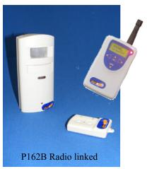
On detecting motion the wired unit (P162A) can trigger a Nurse Call system via the normal wall socket, whereas The P162B can trigger an alarm via secure radio on the P137 and P138 Pagers.
