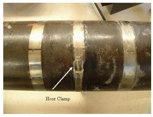
Figure 2. Photograph of the MsS strip secured with a hose clamp for heat treatment
