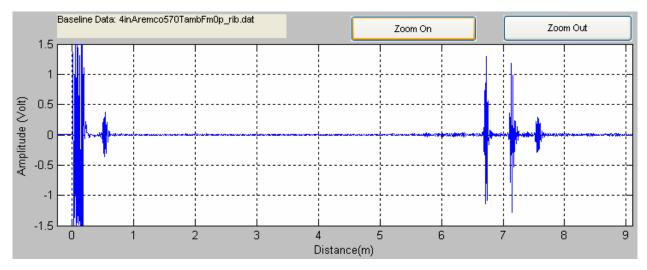
Figure 4. Sensor quality inspection data taken on the 4-inch pipe with the sensor bonded with Aremco 570. Minimal noise is returned from the pipe and the end wall indications are narrow, showing no ringing.
