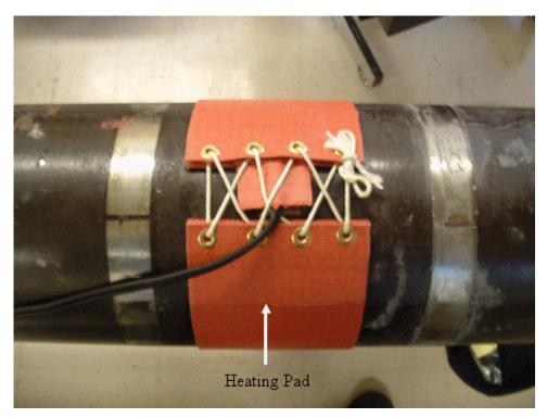
Figure 3. Photograph of MsS strip wrapped in Watlow heating pad
