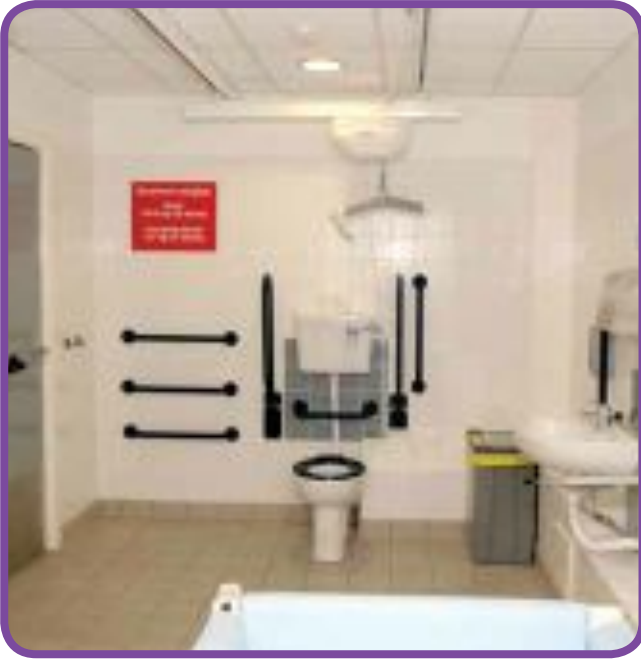
Three horizontal grabrails were incorporated into the design after consultation
