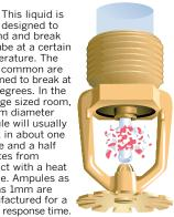
The plug is forced out by the pressurized water behind it and deflected away by a beveled edge. The water sprays over the deflector plate which is designed to distribute it in an even pattern. Water will continue to flow until the main valve is shut off.
