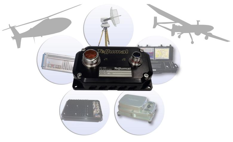
Tellumat's HC-1000 Health and Control Unit provides the health monitoring and control interfaces that are not catered for in a standard UAS autopilot or flight mission computer. The HC-1000 receives commands and provides status values directly to the autopilot or FMC via a RS422/485 serial bus.
