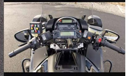
With its standard high-output alternator, tighter turn radius, dedicated wiring harnesses and separate battery for all add-on police equipment, the Concours 14 ABS Police motorcycle supports most equipment packages specified by purchasing agencies.
