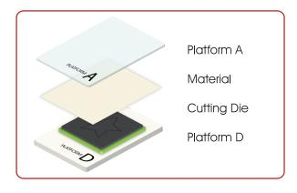
TIP: Never place Platform B or any of the shims or mats as the very top or bottom of the platform combination.
