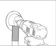
Drill through paste or foam or use a plastic cowl and a Class H vacuum cleaner. A hand drill creates less dust. If you have to use an electric drill, put it on the slowest setting.
