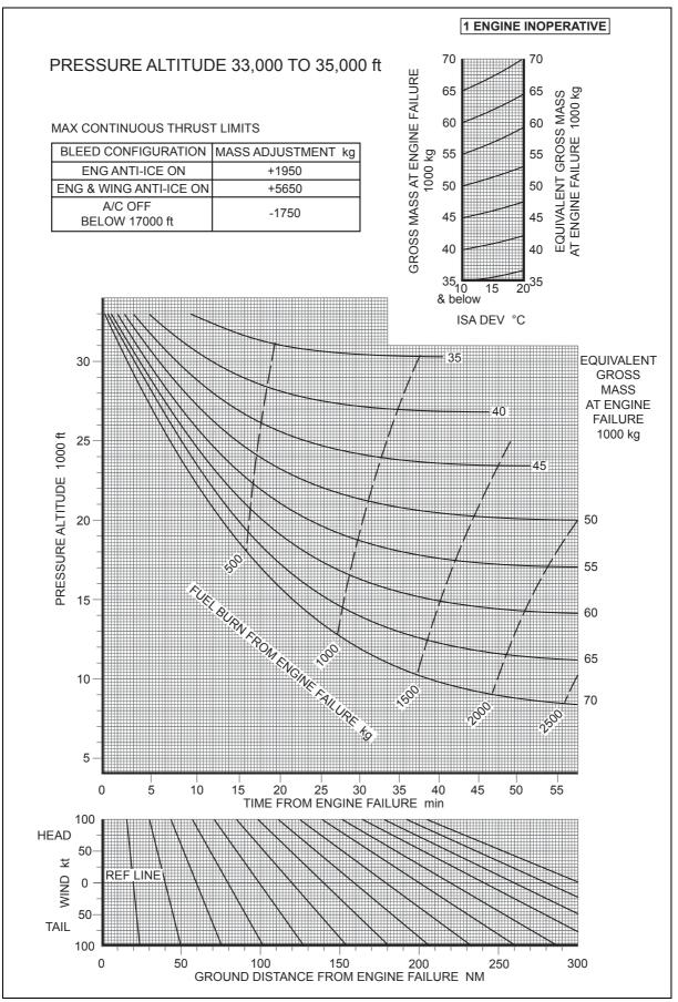
Figure 4.25 Driftdown Profiles – Net Flight Path
