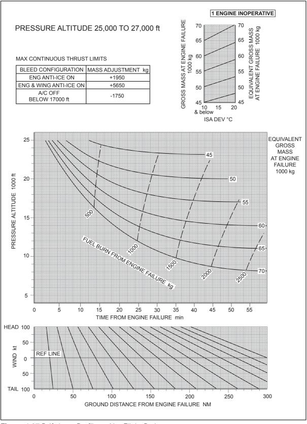
Figure 4.27 Driftdown Profiles - Net Flight Path
