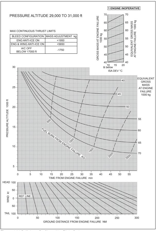
Figure 4.26 Driftdown Profiles – Net Flight Path
