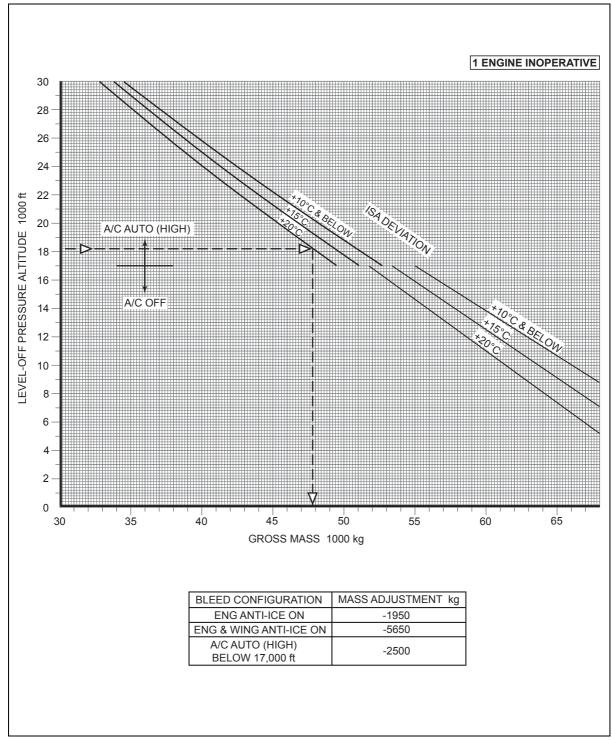
Figure 4.23 Net Level-Off Altitude
