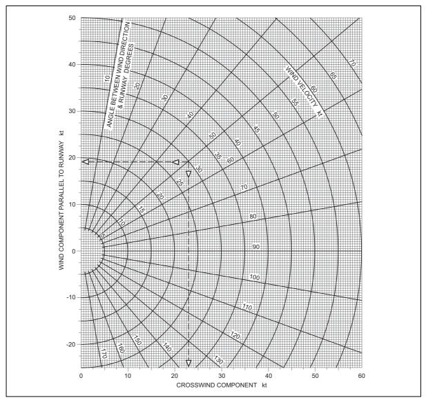
Figure 4.1 Wind Components for Take-Off and Landing
