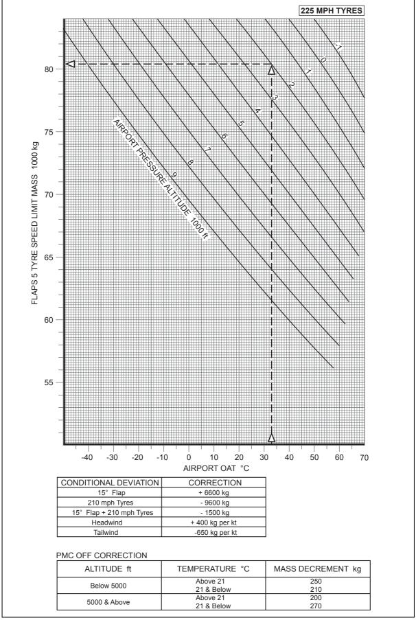
Figure 4.6 Take-Off Tyre Speed Limit
