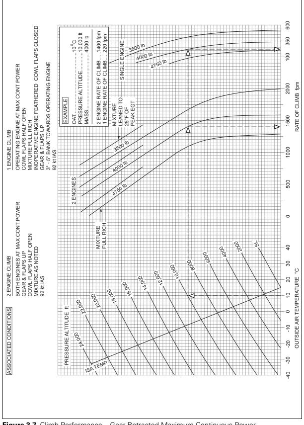
Figure 3.7 Climb Performance – Gear Retracted Maximum Continuous Power
