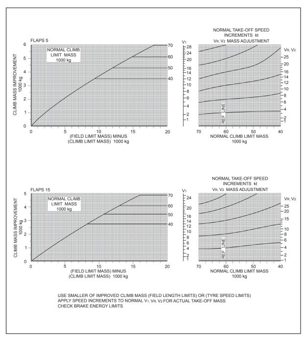
Figure 4.15 Improved Climb Performance – Field Length Limit
