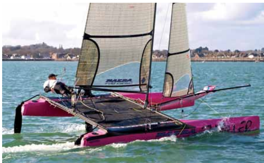
ABOVE You don't need to shift weight right forward when driving upwind due to a combination of hull length, volume and lift from the curved foils.
