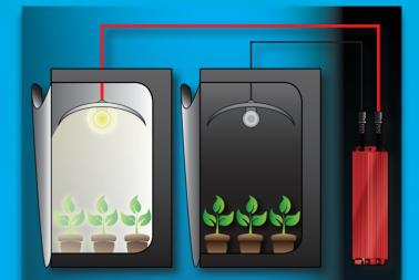
Use the Duo 12 hour FLIP / FLOP setting to run 2 grow rooms on an alternating 12 hour cycle
