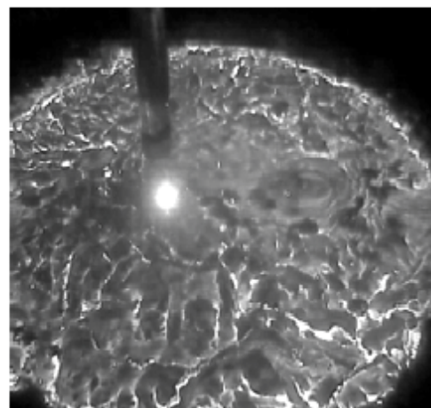
LIBS analysis of liquid slag. Courtesy Dr Cord Fricke-Begemann
